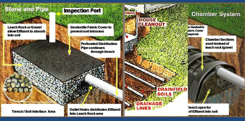
Alternative Systems are used when site/soil conditions <u>DO NOT</u> meet the design criteria for conventional septic systems.
